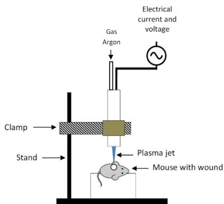
Figure 1: Plasma treatment experimental set-up
