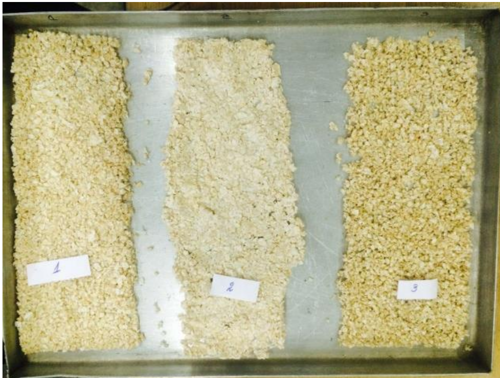
Figure 1. Hydrolysates after vacuum freeze drying: 1 - hydrolysate obtained by enzymatic hydrolysis; 2 - hydrolysate obtained by hydrothermal method; 3 – hydrolysate obtained by chemical hydrolysis (with acids and alkalis).
